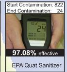
ATP Testing is a CDC recommended monitoring system for evaluating environmental cleaning. ATP measures residue before and after cleaning
